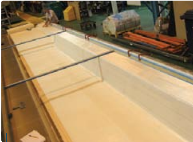
One of the three relatively inexpensive sheet-steel tools used to mold the trailer bed is layed up with the first ply of glass/cPBT prepreg. ■
